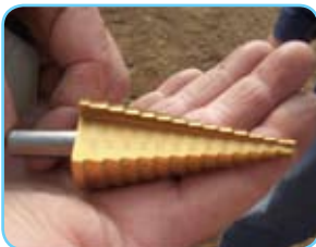
Unibit or tapered drill bit
